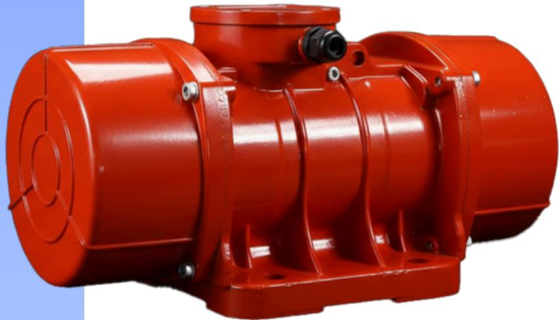
Vibro Motors (or External Vibrators) are specialized asynchronous motors designed to generate centrifugal force through the rotation of adjustable eccentric weights mounted on both ends of the shaft. Unlike standard induction motors that aim for smooth rotation, these units are engineered to create controlled mechanical vibrations for material handling and processing.
